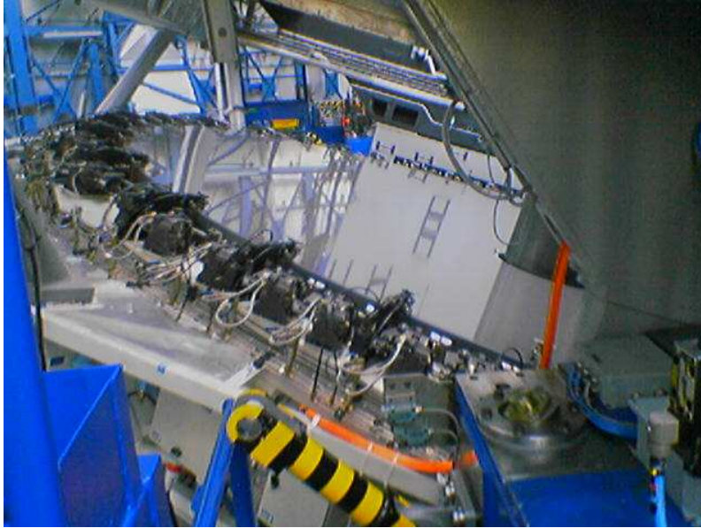
Figure 5.1: The primary mirror of UT2, one of the 4 8.2m telescopes of the VLT, seen from the Nasmyth platform.
