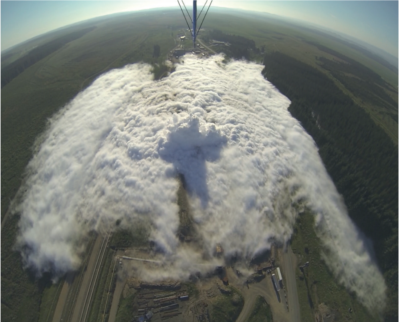
Figure 4-2 Aerial Photograph of a CO 2 Pipeline Fracture Test at DNV Spadeadam
