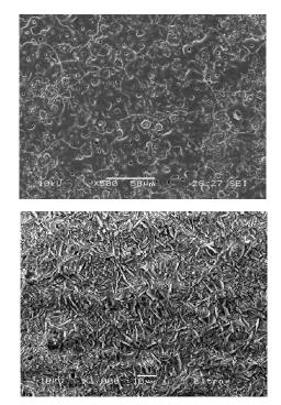
Figure 2. Anodized magnesium alloy coatings. Top: Amorphous coating. Bottom: Crystalline coating.
