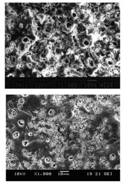
**Figure 1.** 1000X SEM images of the surfaces of anodized ZE41 magnesium alloy. Top: Coating produced by the Tagnite process.\* Bottom: Coating produced by Eltron's low-cost process.
