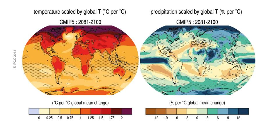
Change at each grid point for a 1°C change in Global Mean Temperature
