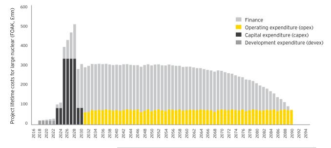
Figure 2 - Breakdown of un-discounted lifetime costs for a general FOAK large reactor<sup>4</sup>
