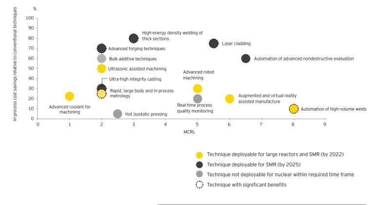
Figure 15 - The in-process savings for each technique against the maturity of the process
