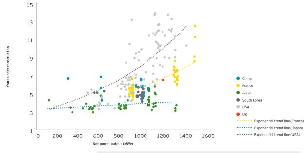
Figure 11 - Effects of size and approach on large reactor (PWR) construction schedules<sup>20</sup>
