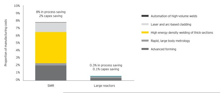
Figure 14 - The potential in-process savings through implementation of advanced manufacturing techniques<sup>H</sup>
