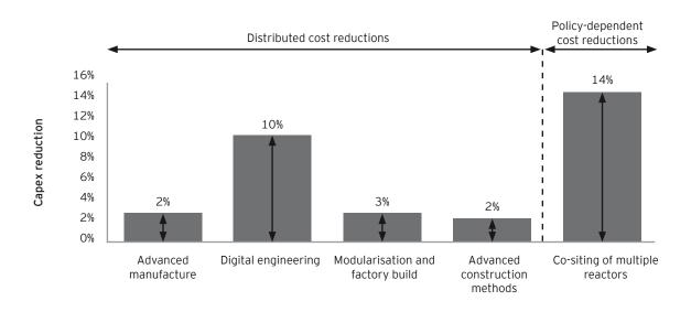
Figure 12 - The potential capex reduction through applying different techniques to SMR<sup>F</sup>
