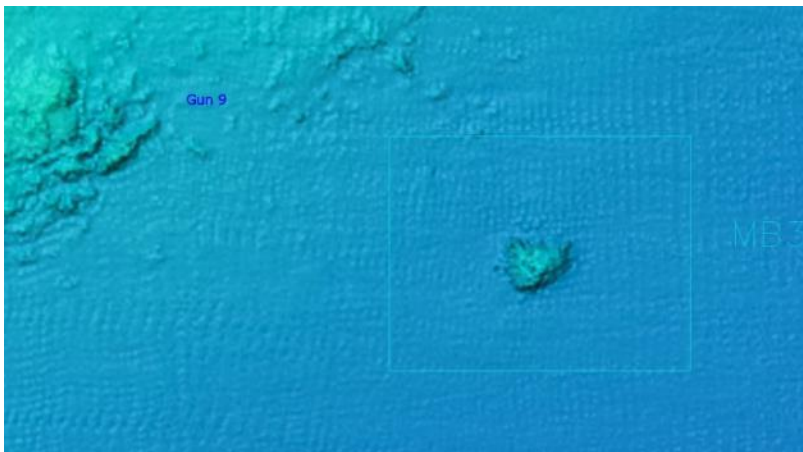
Fig 10 A detail from the 450 mHz MBES survey of Colossus showing a small jagged target in the vicinity of gun 9.
