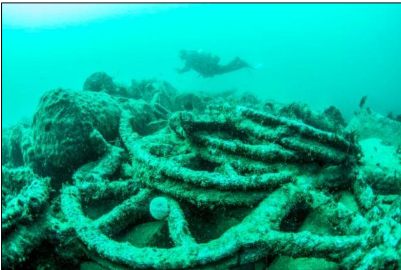
Fig 16 A seabed-level view of some of the sheave wheels on the north- east corner of the cargo mound. The wheels are 1.15m in diameter. The cylindrical object on the left is a windbore – the bottom section of a set of pump pipes.
