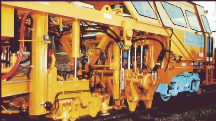
A self-propelled tamping and lining machine used for track maintenance.
