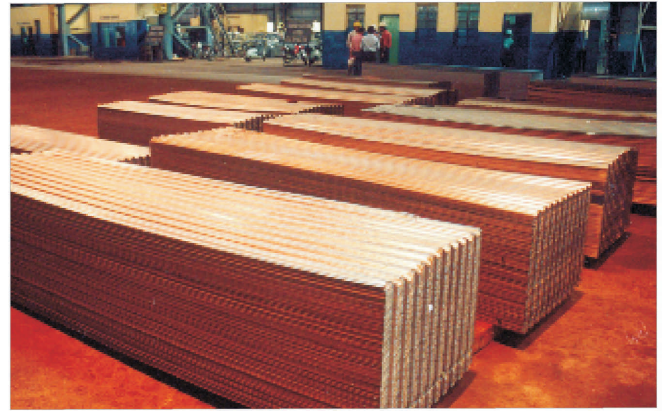
Galvanised corrugated sheets are used for roofing
