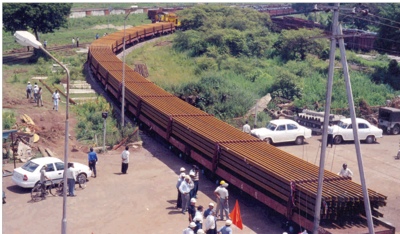
Long rails loaded on wagons for despatch
