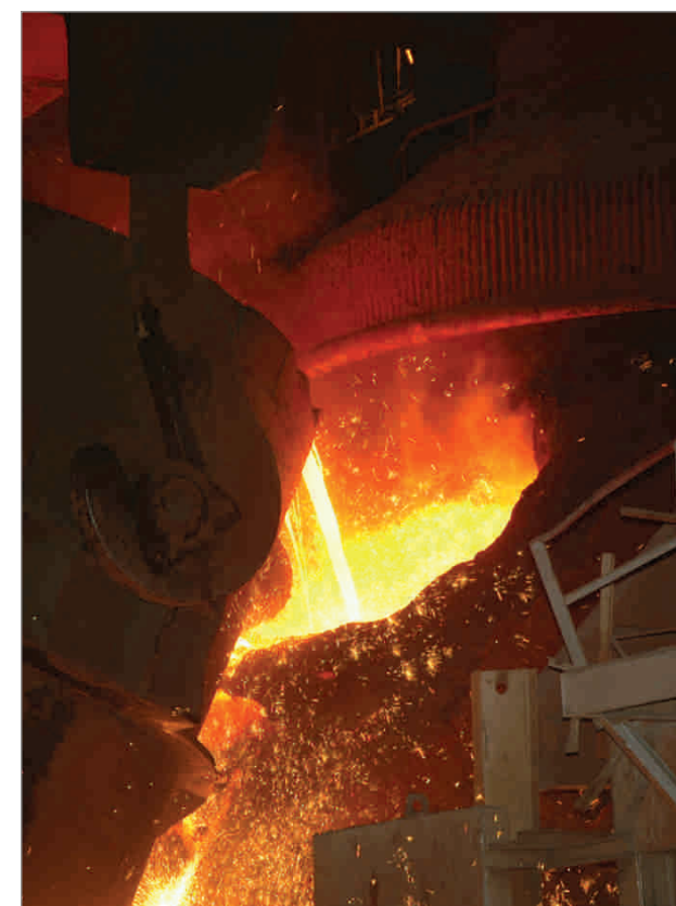
Anti-clockwise from top: Hot metal being poured into a ladle; then treated at a Basic Oxygen Furnace; and finally cast into saleable steel
