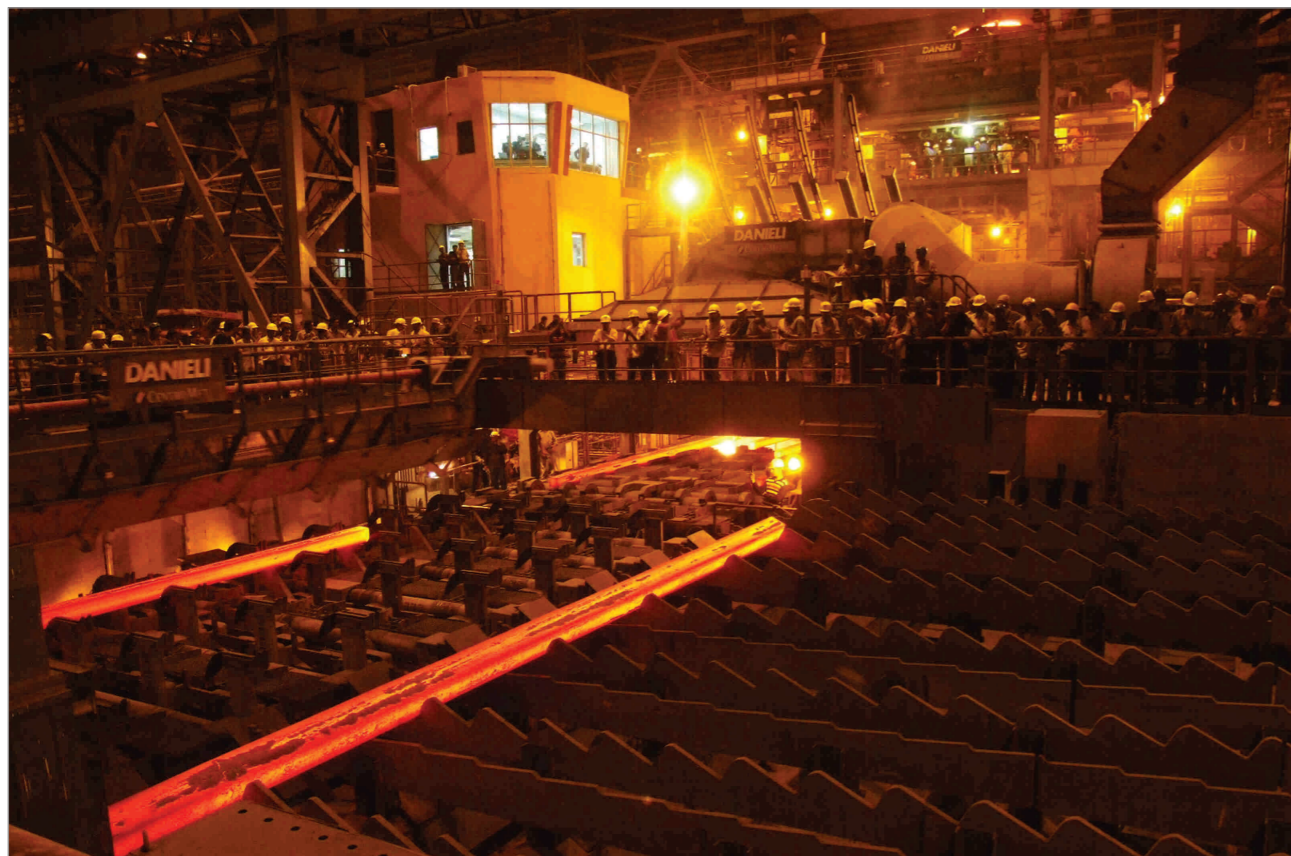
The newly installed bloom caster in operation at Durgapur Steel Plant
