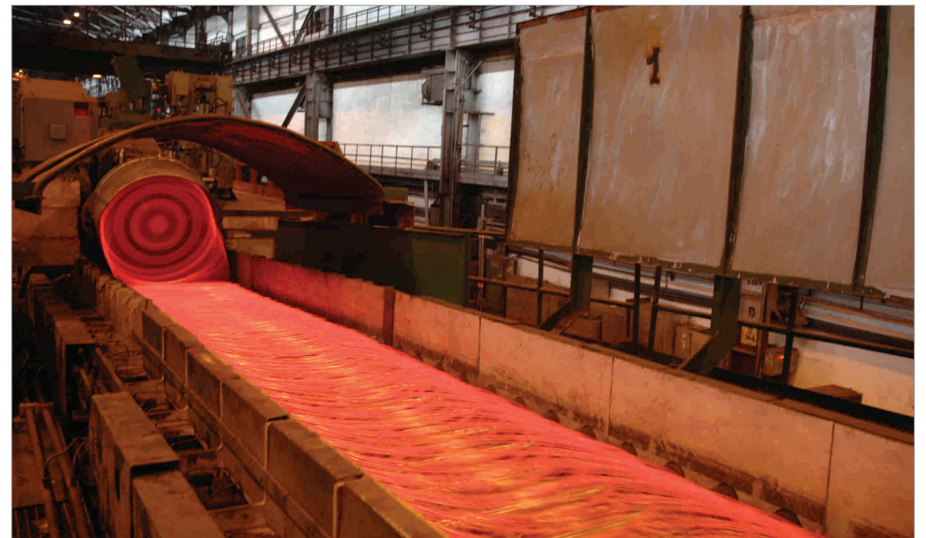
Wire rod being rolled from the modern 'B' strand of Wire Rod Mill
