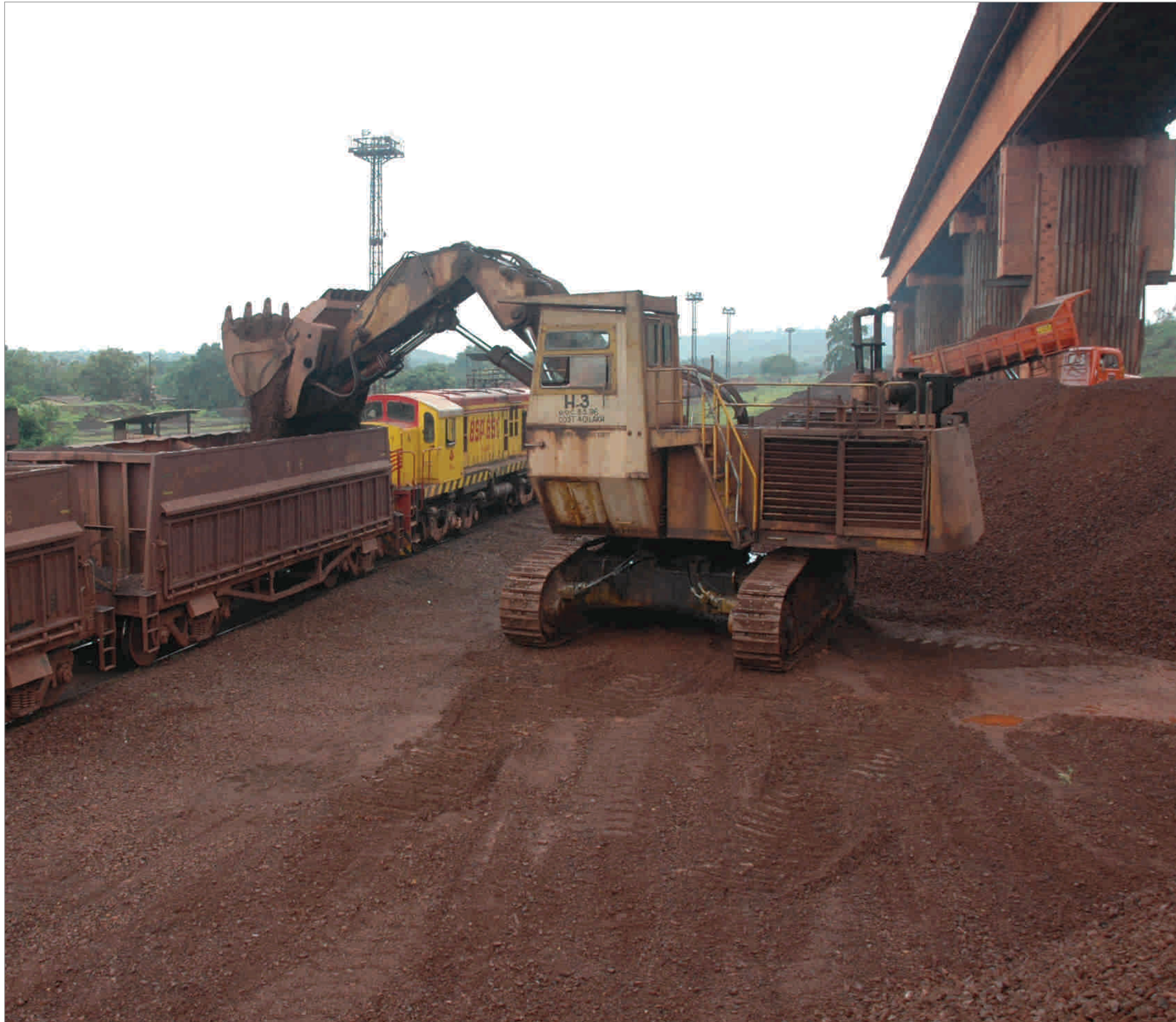
This is where the steel making process begins: Iron ore being despatched from a mechanised mine
