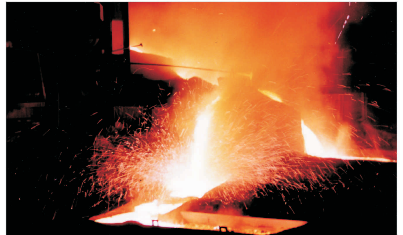
A view of tapping of liquid ferro alloys from submerged arc furnace
