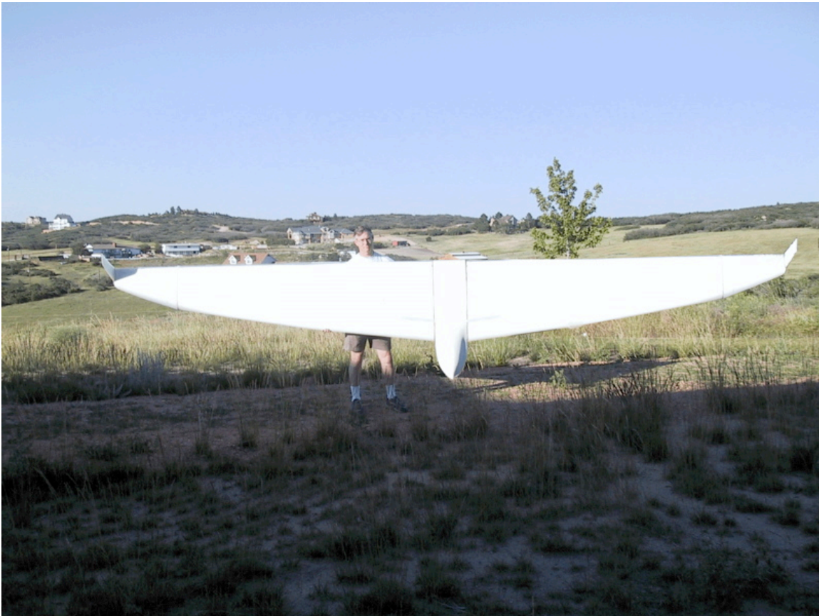
21 foot wingspan Mars glider. Payload capacity (remote sensing instrumentation, etc.) of several Kilograms
