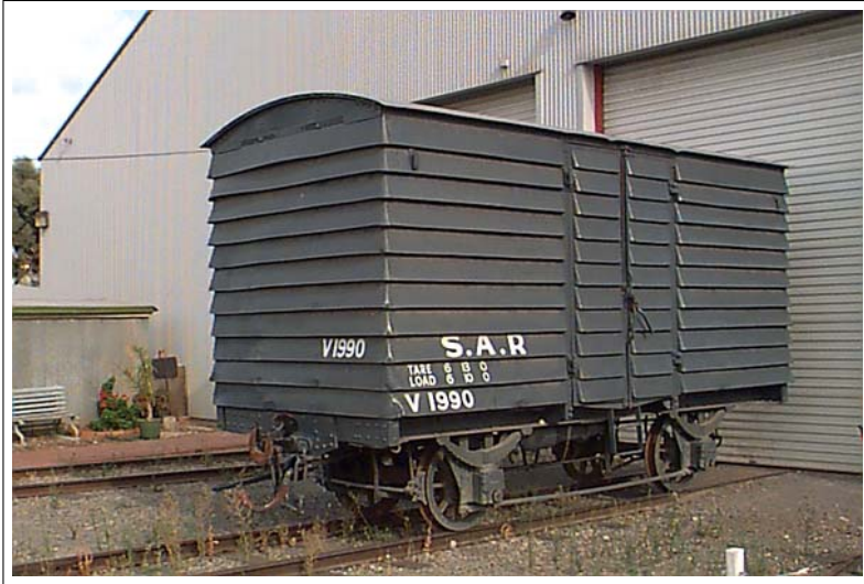
South Australian Railways - V Class Steel 4-wheel Louvred Van No. 1990 (NRM Collection)
