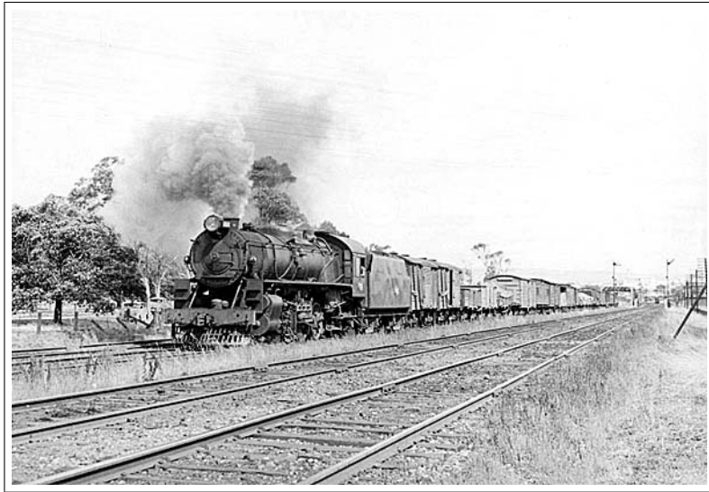
South Australian Railways - 700-class 2-8-2 steam locomotive No. 702 - Northbound Dry Creek transfer freight locomotive 702 at Torrens Bridge. 8.12.1956 ( D.Colquhoun )
