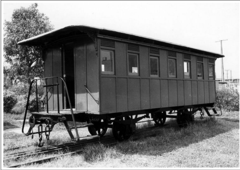
South Australian Railways - 4-wheel 2nd-class Saloon Car with end platforms - No. 3 prior to full restoration ( Murray Billett )
