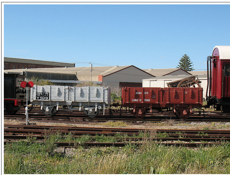
South Australian Railways - Y Class 4-wheel Open wagon (drop-sides) Nos.5019 and identical except for livery NGSA 373 - 21st September 2008( Chris Drymalik )
