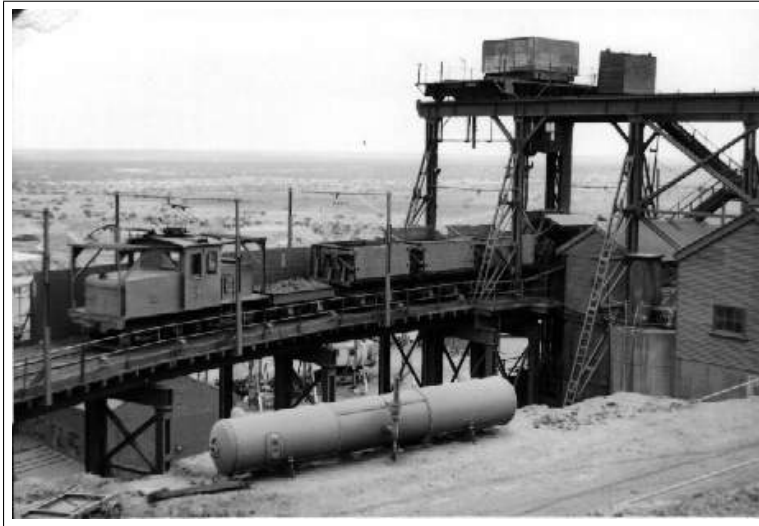
Broken Hill Proprietary Co. - Iron Knob Tramway - Electric Locomotive No. E1 - Metro-Vickers built, BHP electric loco No. 1 goes about its business at BHP smelter Whyalla ( NRM Collection )
