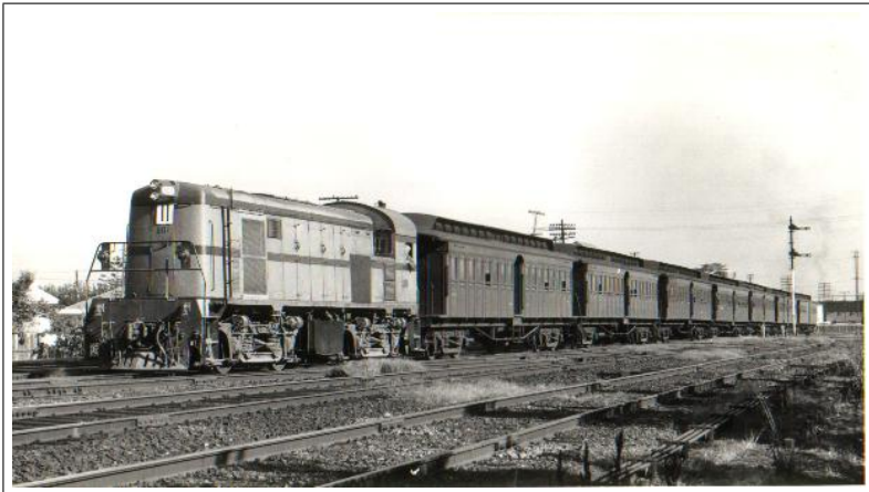
South Australian Railways 800-class Bo-Bo Diesel Electric Locomotive No. 801 hauling a suburban passenger train ( NRM Collection )
