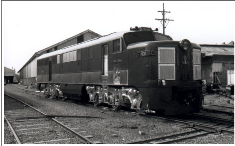
South Australian Railways - 900-class A1A+A1A diesel electric locomotive No. 900 Lady Norrie 20.10.1988 ( R.E.Fluck )
