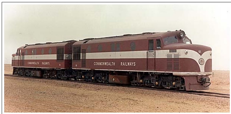
Commonwealth Railways - NSU-class A1A-A1A Diesel-electric locomotive No. 61 - NSU 61 and NSU 56. - circa 1960s ( Commonwealth Railways )
