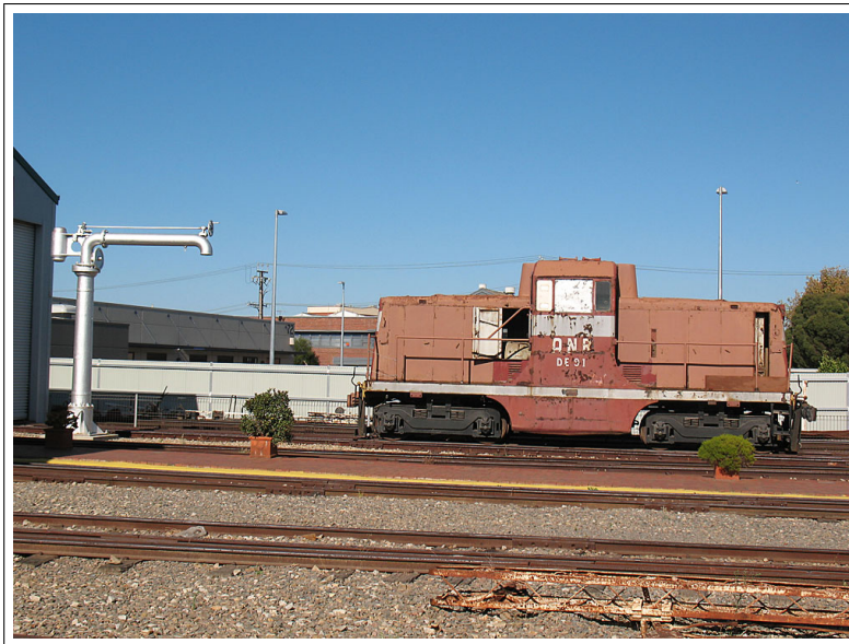
Commonwealth Railways - DE-class Bo+Bo diesel-electric locomotive No. 91 sits alongside a CR water column - 2nd April 2010 ( Chris Drymalik )
