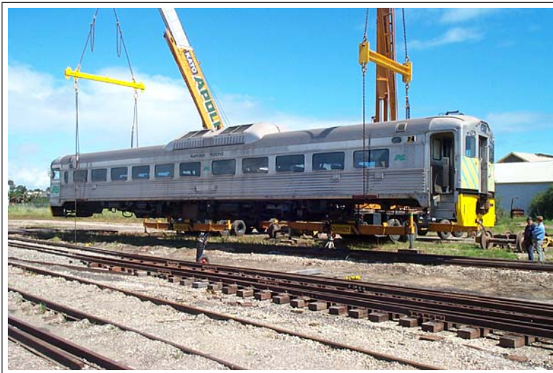
Commonwealth Railways Budd Railcar CB 1 being placed on it's standard gauge power bogies - 3.10.2001 ( Chris Drymalik )
