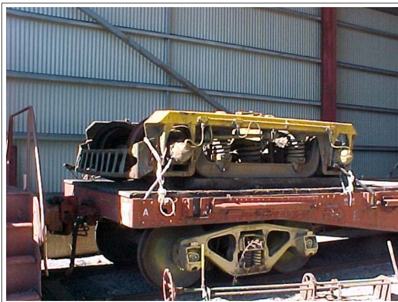
Commonwealth Railways - Budd Railcar CB 1 - One of the standard Gauge bogies from CB 1. - 18 April 2000 ( Chris Drymalik )
