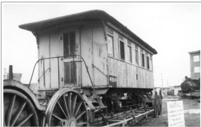
South Australian Railways - 4-wheel 2nd-class Saloon Car with end platforms - No. 3 at Mile End Railway Museum on the crocodile wagon - at this stage it was still numbered '4884' - 25.9.1969 ( R.E.Fluck )
