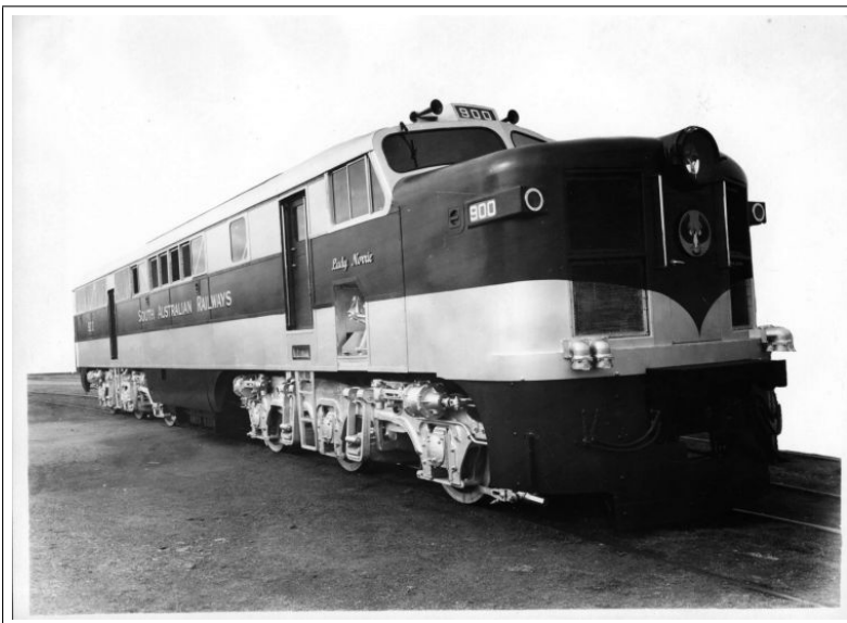
South Australian Railways - 900-class A1A+A1A diesel electric locomotive No. 900 Lady Norrie - Loco 900 as built in red/silver livery posed at the Islington Workshops in 1951 ( NRM Collection )
