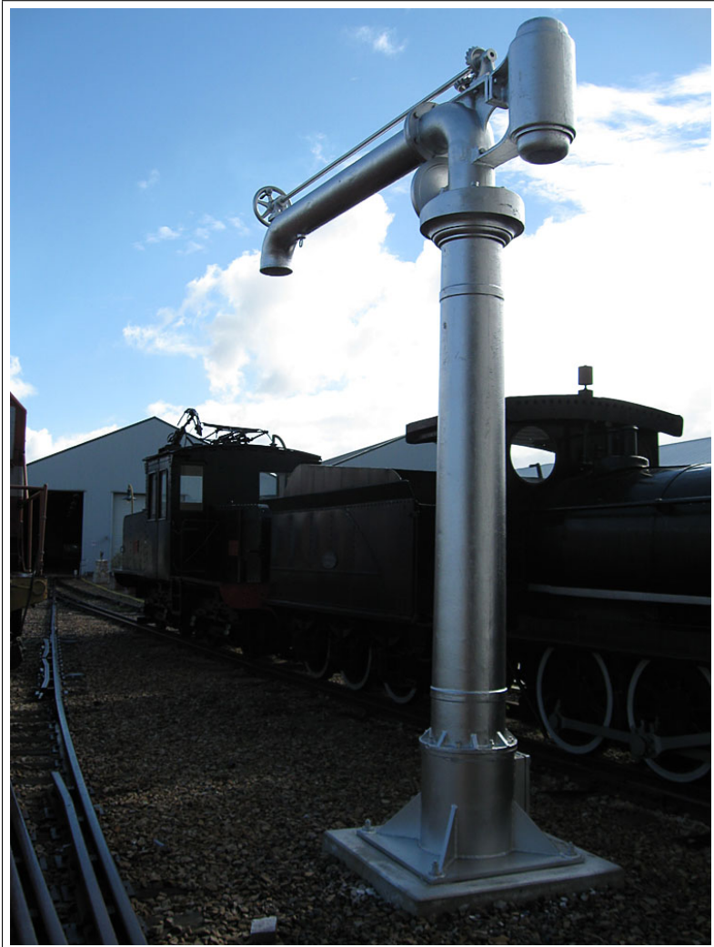
A Commonwealth Railway water column sits sanswitched between engines in front of the Fluck Pavilion - 27th July 2008 ( Chris Drymalik )
