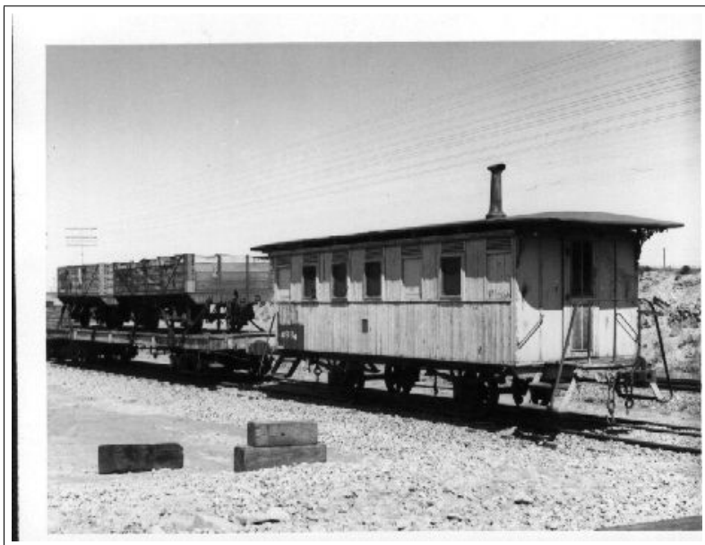
South Australian Railways - 4-wheel 2nd-class Saloon Car with end platforms - No. 3 (as No. 4884) at Peterborough prior to delivery to the Mile End Museum ( Ken Wicker )
