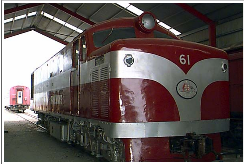
Commonwealth Railways - NSU-class A1A-A1A Diesel-electric locomotive No. 61 ( NRM Collection )
