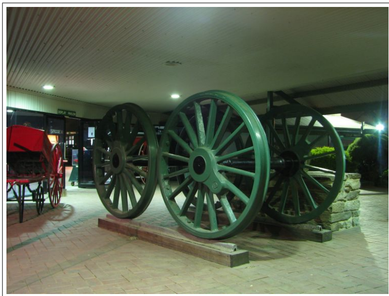
Locomotive wheels originally used on 2-4-0 Tank Locomotive 'Adelaide', 'Victoria' or 'Albert' ( A. Peters )
