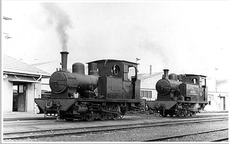
Broken Hill Associated Smelters, Port Pirie - 0-6-0 tank locomotive Peronne . Locos Peronne & Pt Pirie in smelters yard at Port Pirie, 1959 ( D. Colquhoun )
