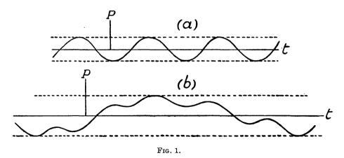
Suppose the correlation coefficient between p and  $d^2p/dt^2$  is small, but that the standard deviations of dp/dt and  $d^2p/dt^2$  are the same as in curve (a), Fig. 1, then the slopes and curvatures will be of the same magnitude
