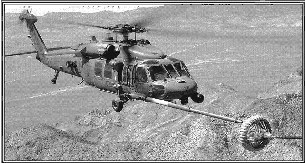
Figure 268: NELLIS AIR FORCE BASE, Nev. (AFIE) -- An HH-60G Pave Hawk from 66th Rescue Squadron here refuels from an MC-130E Combat Talon from the 711th Special Operations Squadron at Duke Field, Fla., on Aug. 5 during Millennium Challenge 2002.
