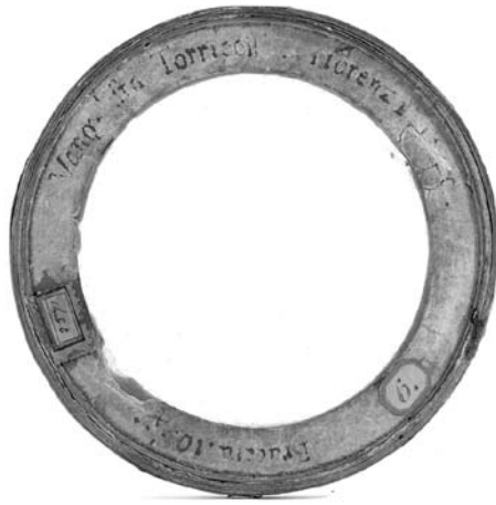
Ill. 9. Telescope objective of Torricelli in Florence (Museo Galileo, Inv. 2571).
