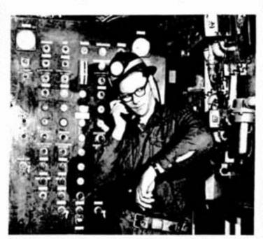
This is the control centre that handles loading of the two skips operating in Frood-Stobie No. 9 shaft. A fully automatic system, it can be switched to manual operation if required. Pressure-sensitive electric load cells control the flow of ore to the station's two 400-cu.-ft. measuring boxes which dump into the skips. Skiptender Lorne Palmer is seen checking the hoisting schedule with the hoistman.
