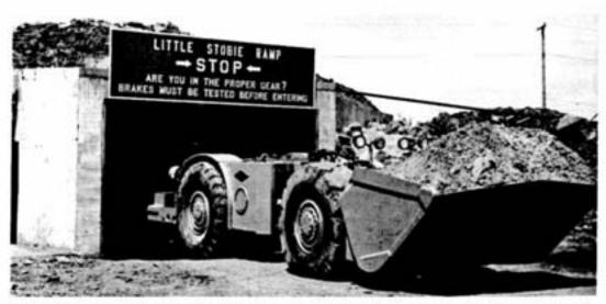
Entering the mine portal and heading down the ramp, this husky load-haul-dump machine is carying a 7-ton load of crushed rock that will be used for road bed. Driven at an incline of 20%, the ramp is 16 feet wide and 12 feet high. Now down to the 600 level, the winding road is 3,250 feet long.
