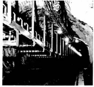
Nearly a mile long, this 42-inch roof-suspended conveyor is located on the 2400 level and carries are from Little Stable Mine to Frood-Stable No. 9 shaft. With a belt speed of 481 feet per minute, it can deliver 1,000 tons of muck per hour. It is powered by a 250-h.p. motor. The endless belt has a total length of 9,400 feet, weighs 1,034 tons, and carried a price tag of close to \$200,000.
