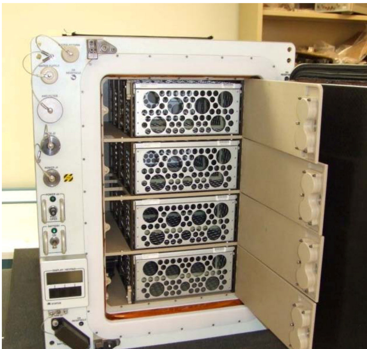
GLACIER , a freezer for transportation and preservation of samples, will be carried on the middeck of Atlantis.
