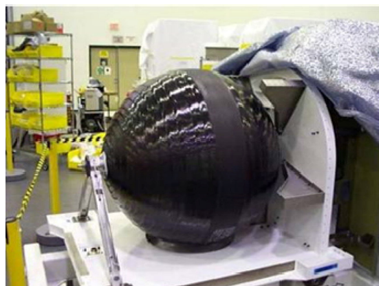
High-Pressure Gas Tank (HPGT) with the cover removed.
