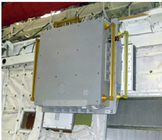
PEC 7A installed on Orbiter Sidewall.
