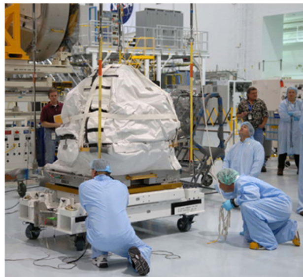
Boeing technicians prepare to load a CMG onto an ELC.
