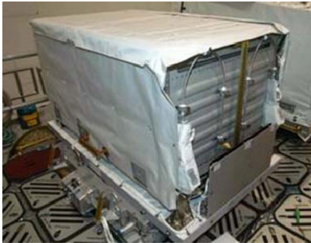
Nitrogen tank assembly installed on the ELC.
