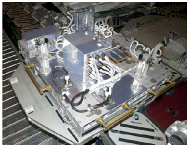
MISSE-7 Support Base installed on ELC2.
