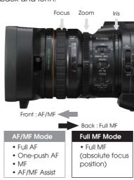
When the focus ring is in the front position, the lens works as an auto focus lens. Either Manual or Auto Focus mode can then be selected using the AF/MF switch on the lens. When the focus ring is set to the back position, the lens has an absolute focus position.
