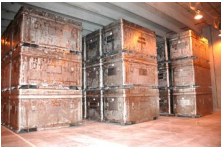
Figure H.2: Bruce Units 1 & 2 Retube Waste Containers currently in storage at the Ontario Power Generation's Western Waste Management Facility (WWMF) Retube Component Storage Building
