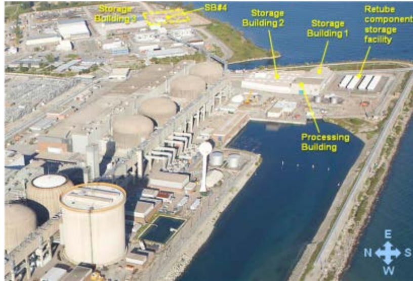
Figure 4.5: Pickering Waste Management Facility, phase I (processing building, storage buildings 1 and 2, retube components storage building) and phase II (storage building 3, future storage building 4) areas
