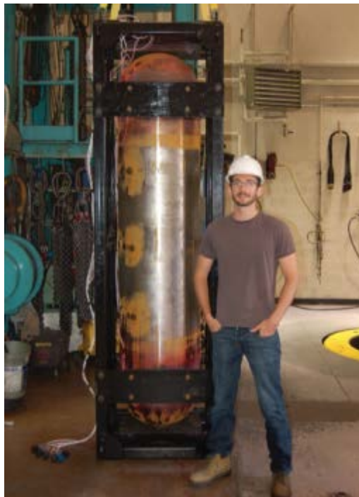
Figure K.4: NWMO staff member with prototype spent fuel container at the Applied Research Laboratory's High-Pressure Test Facility at Pennsylvania State University
