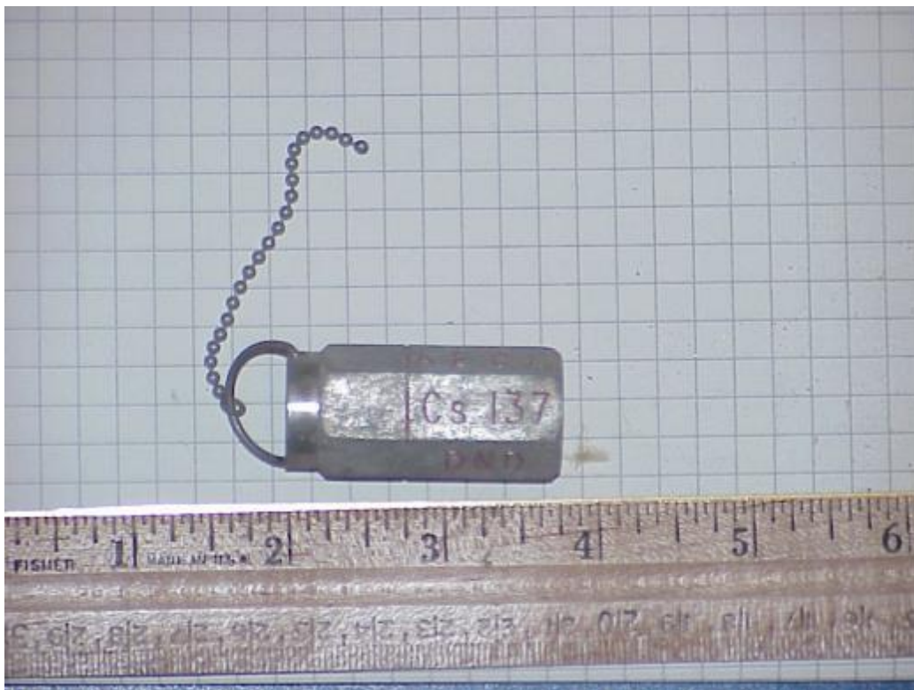
Figure J.1: Cesium-137 radioactive sealed source
