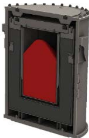
Figure H.3: Darlington Retube Waste Container (RWC) and Darlington Storage Overpack (DSO) cutaway drawing that shows the storage configuration (RWC inside the DSO)
