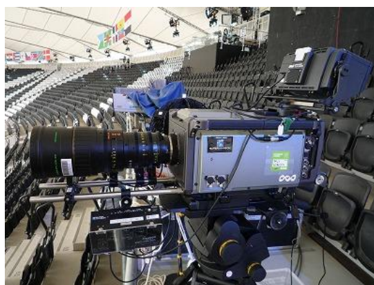
FIGURE 54 1.25-inch 4-CMOS camera and 5x lens
