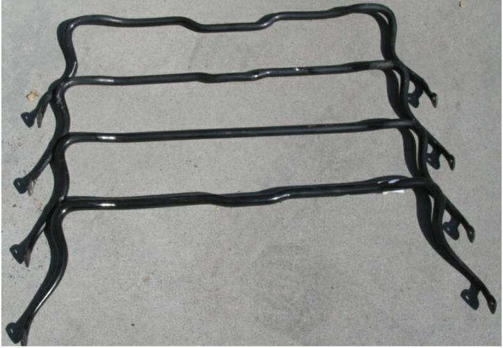
Part# 31 35 1 131 620 (far right) anti-sway bar arms are <sup>3</sup>/<sub>4</sub> inch longer as illustrated below and were used on subframes <u>without</u> the "X" frame stiffener that was introduced on models produced after 4/92,
