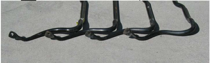
Part# 33 535 1 131 620 is on the right side, also has an exaggerated and longer "turn-up" at the end to clear tie rods. If aftermarket manufacturers don't follow this outline and arm length, interference with steering and suspension components may result.
