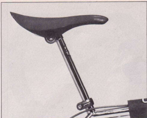
An Aero MX seat was used along with CW chromemoly seat post and a Shimano DX seatpost clamp.
