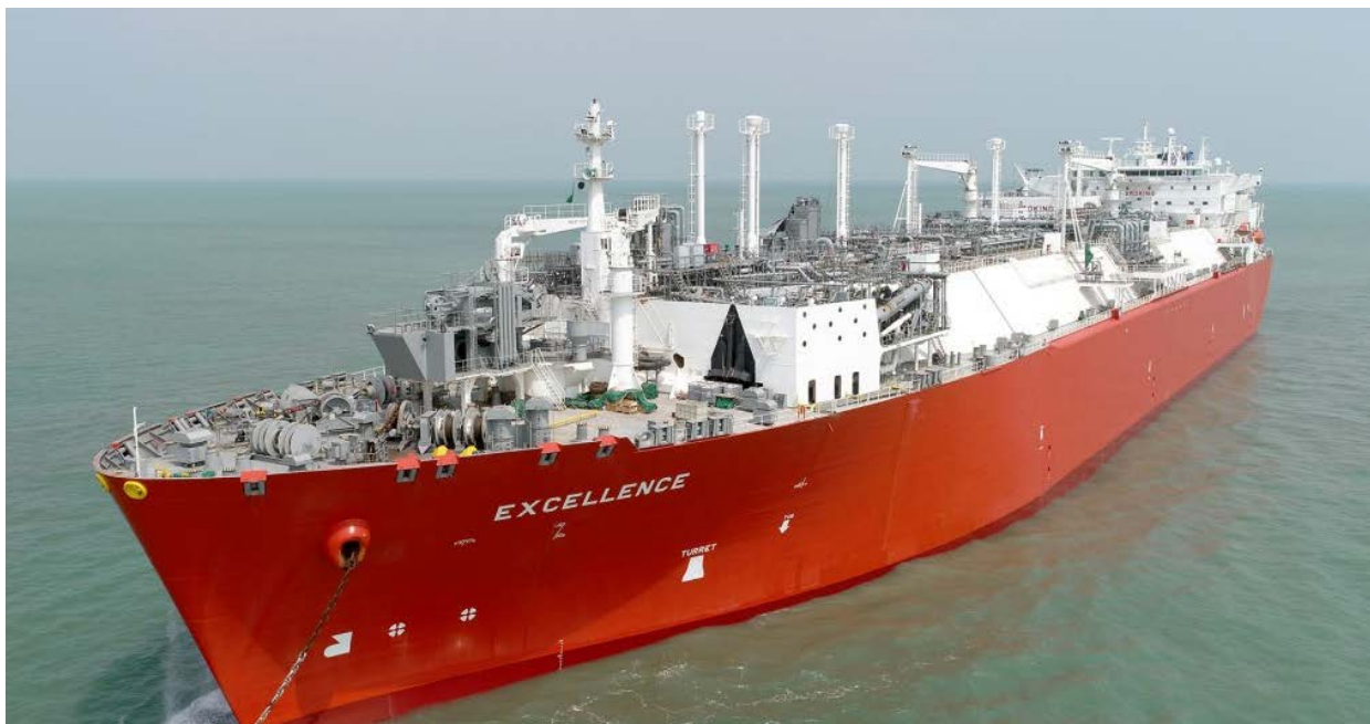
Excelerate Energy Bangladesh Limited (EEBL) FSRU
