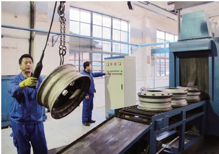
■ 零件清洗机及配套污水处理设施 Component cleaning machine and ancillary wastewater treatment facilities
