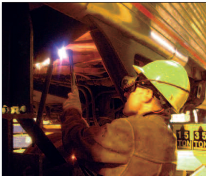
Photo: Joseph P. Riley Car Repairman Kenneth A. Dalton cuts a vertical shock arm as part of a Level Three overhaul on an Amfleet I coach at Bear Car Shops in Delaware.
