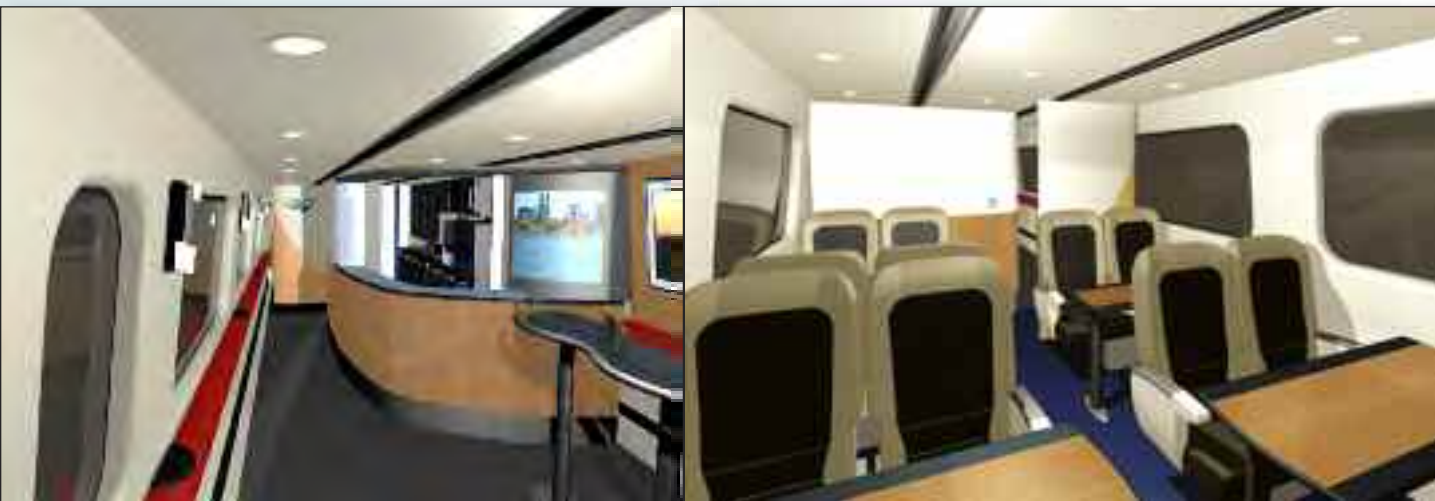
The updated café car maintains a distinct food service area while creating 27 new seats, including table seating, at the other end. The food service end of the car includes an open floor layout that provides ample space for passengers to wait in line without disturbing those in the new revenue seating at the opposite end of the car.
