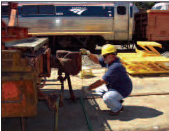
Photo: Stephen Reader Repairman/Inspector Jim Ricchiuti measures the coupler while checking a tie car at Bear Maintenance Facility.
