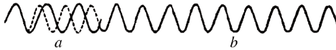
Figure 6. Measured waveforms of the time dependence of (a) ac current of the Straßburg power station, (b) tuning fork oscillation 37 .
