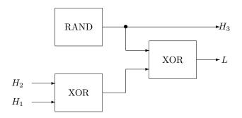
Figure 9.4 – insecure composition of secure systems with feedback
