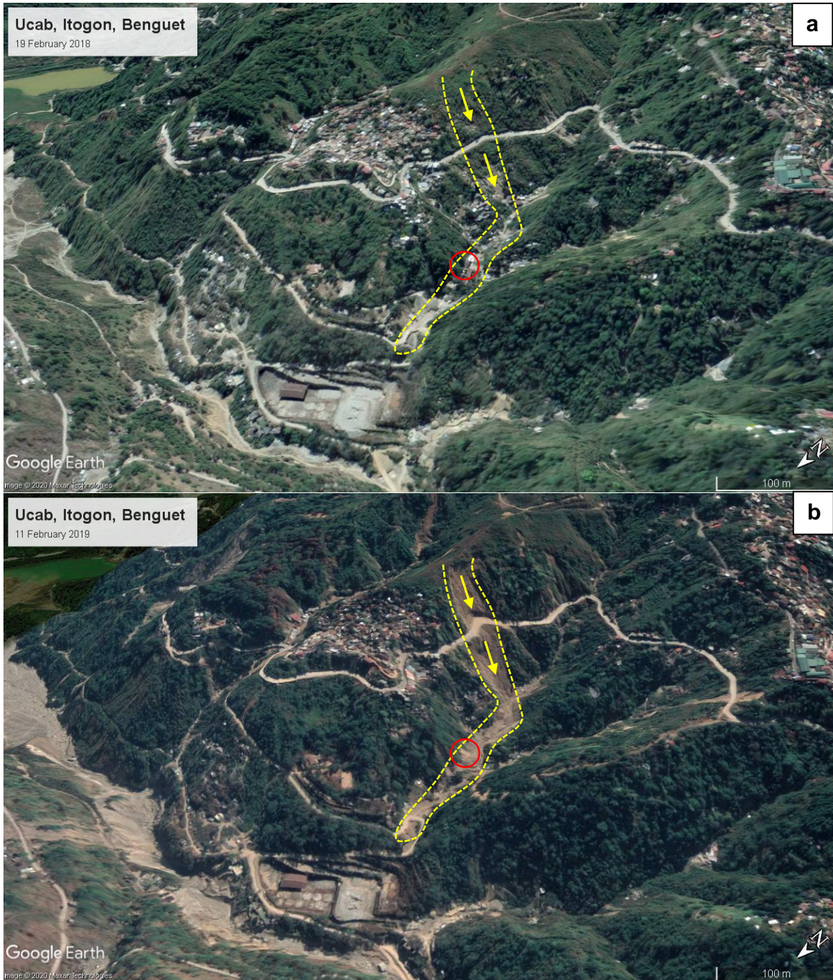
Fig. 5.2. Google Earth images of Sitio First Gate, Barangay Ucab, Itogon, Benguet on (a) 19 February 2018 and (b) 11 February 2019. The debris flow is outlined in yellow while the arrows show the direction of the landslide. The approximate location of the concrete bunkerhouse that was used as evacuation shelter by the miners and their families is encircled in red. In Fig. 5.2b, the Baguio-Bua-Itogon road had already been cleared of obstruction because the image was taken nearly 5 months after the incident.
