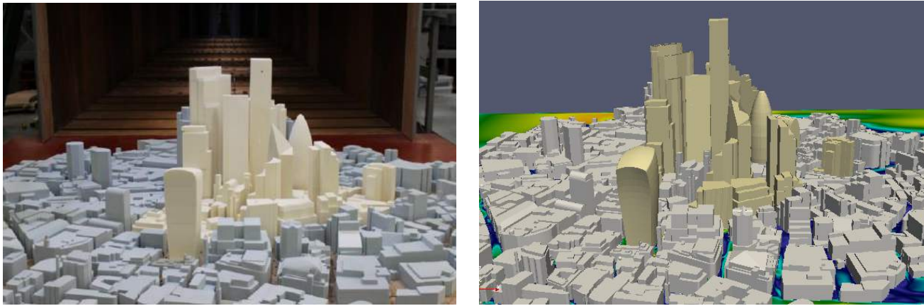
Figure 1. Wind Tunnel Model (left) and CFD Geometry (right)
