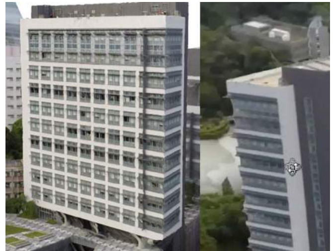
Figure 6. Mesh models of surveyed urban context created with SfM.
