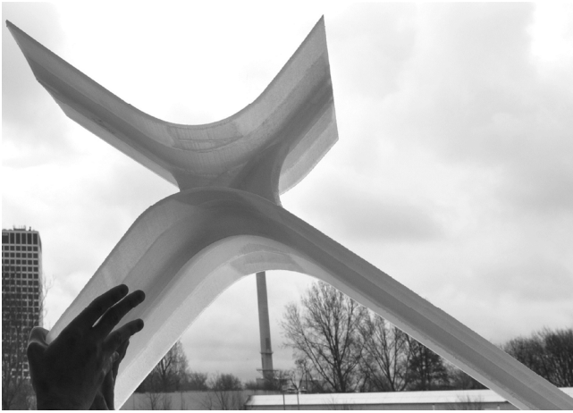
Figure 6. Full-scale 3D-printed prototype: one module.
