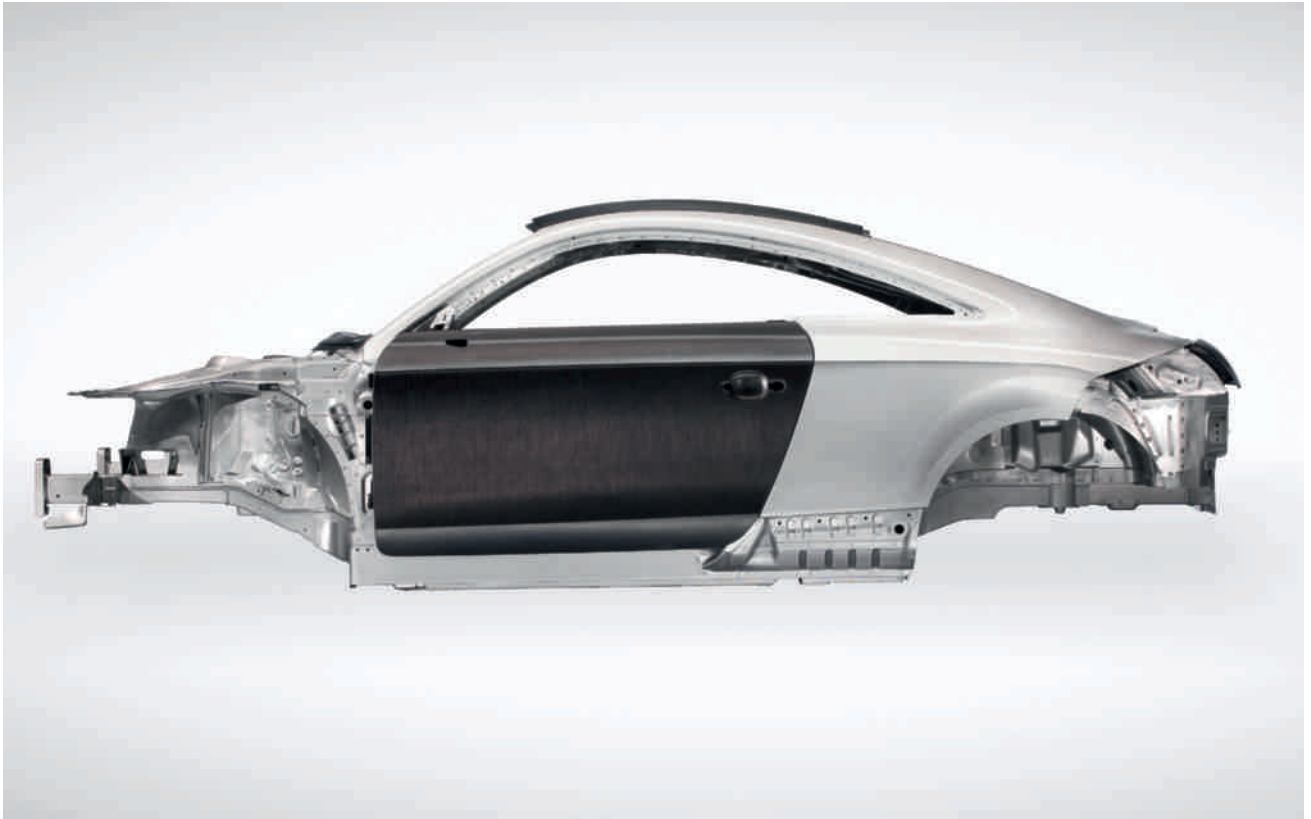
Steel, aluminum, CFRP: The body of the Audi TT ultra concept represents the ideal combination of the materials according to the ultra principle.
