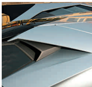
More air! Increasing power requires larger air intakes on the Miura, Countach and Aventador (from above).
