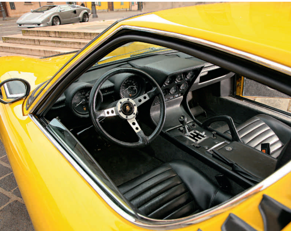
Classic sports car design: the inside of the Miura with gate shifting and large dials.
