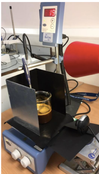
Figure 1: Experimental set up showing a beaker on the temperature-controlled magnetic stirring heat plate.
