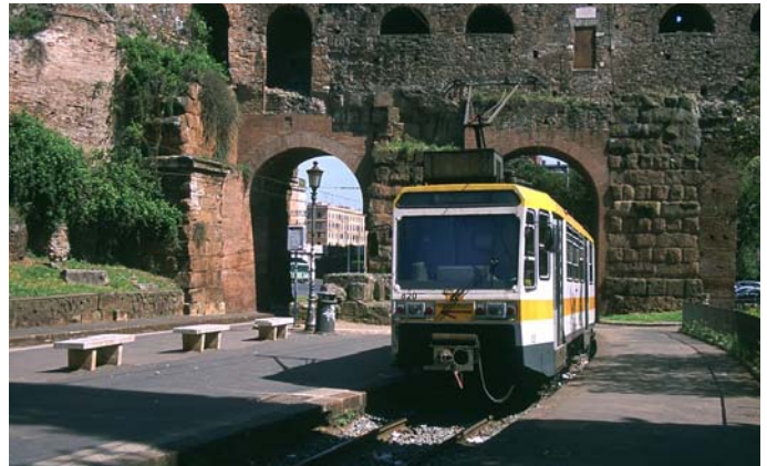
The Porta Maggiore station of Rome's narrow-gauge former interurban line is right under the old Roman walls. Contrast car 106 from the 1920s with car 820 from 1989. Service on the 5-mile-long line, which is electrified at 1,650 volts, is very frequent during rush hours.
