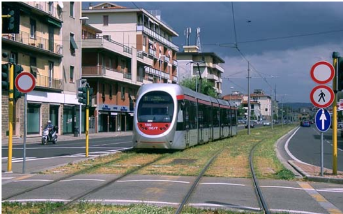
Most of the tramway is located on center-of-the-road reservation. An AnsaldoBreda Sirio car approaches the Talenti station.
