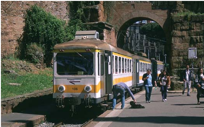
The Porta Maggiore station of Rome's narrow-gauge former interurban line is right under the old Roman walls. Contrast car 106 from the 1920s with car 820 from 1989. Service on the 5-mile-long line, which is electrified at 1,650 volts, is very frequent during rush hours.
