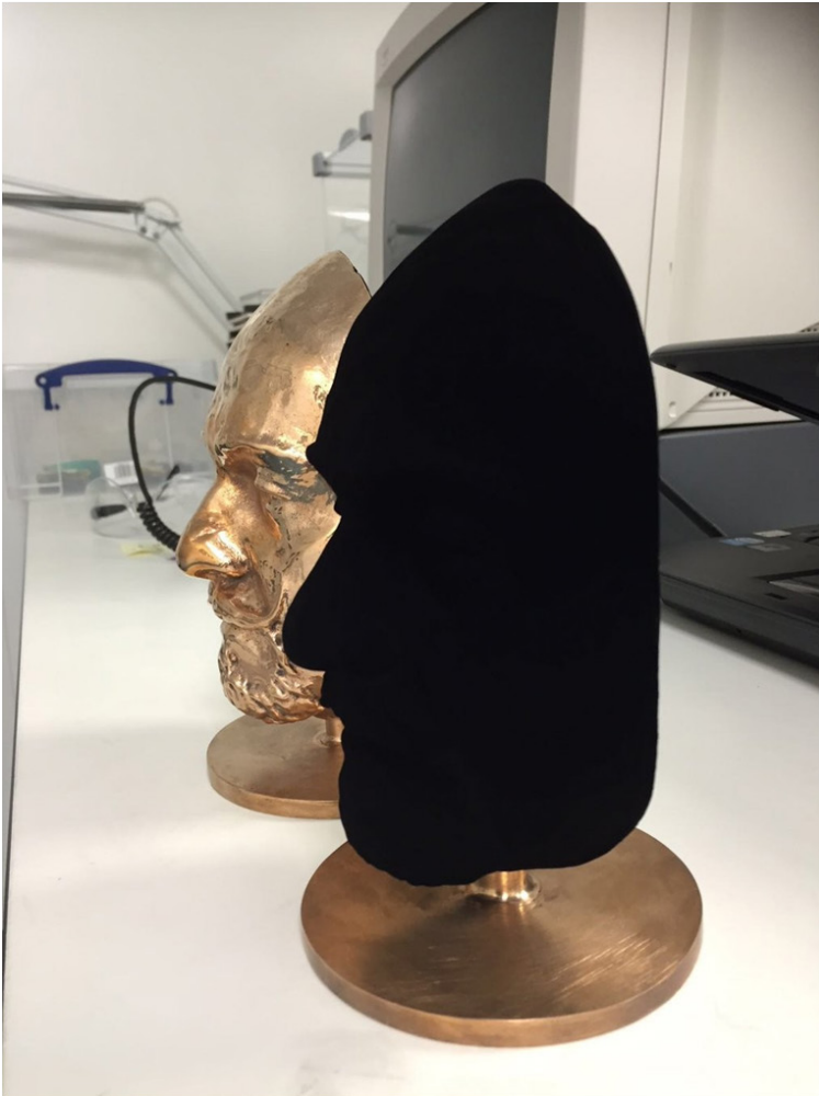
Vantablack S-VIS Coating on a Three-Dimensional Sculpture of a Face. Photo courtesy of Surrey NanoSystems.
