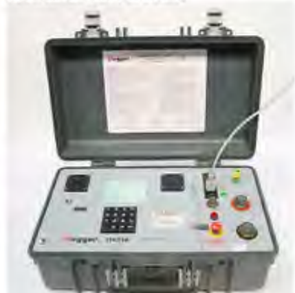
THREE PHASE TRANSFORMER TURN RATIO TESTS
