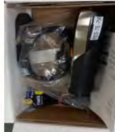
HYGROMETER WITH HYGROMETER PROBE Maker: TESTO Model: 635
