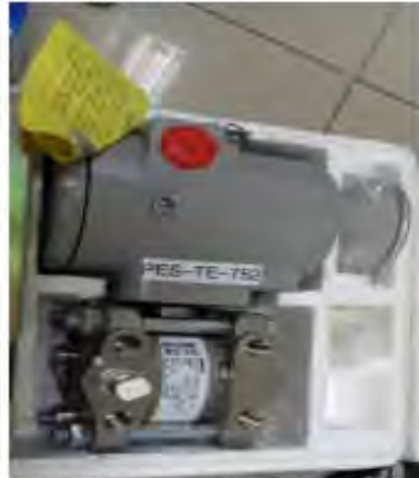
PRESSURE TRANSMITTER Maker: SMAR Model: LD301D-21I-TU10-011/PO/Y2/Y4
