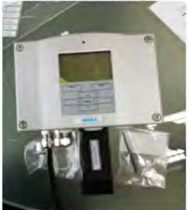
HUMIDITY AND TEMPERATURE TRANSMITTER Maker: VAISALA Model: HMT331
