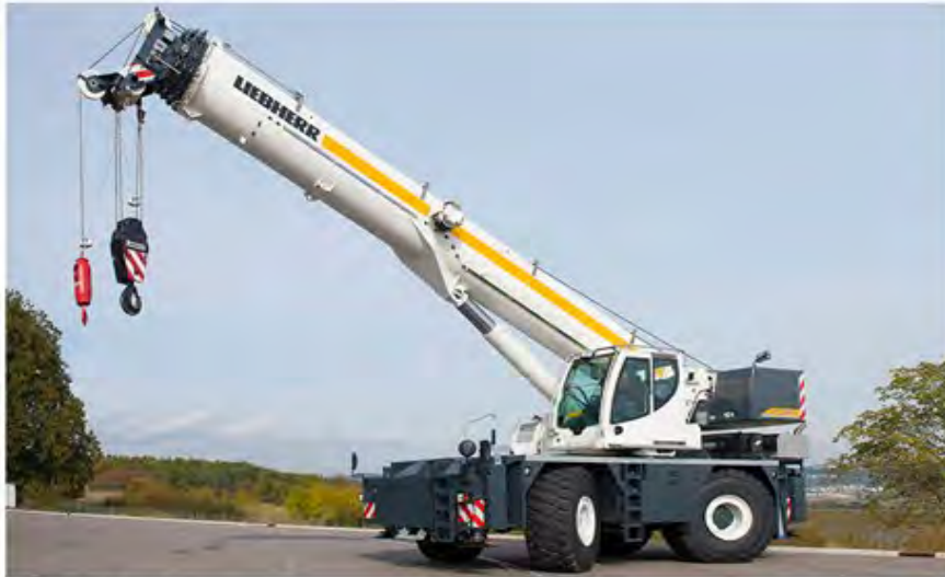
Mobile Crane Model: Rough Terrane 90 tons "Liebherr" "S"
