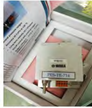
BAROMETER Maker: VAISALA Model: PTB110
