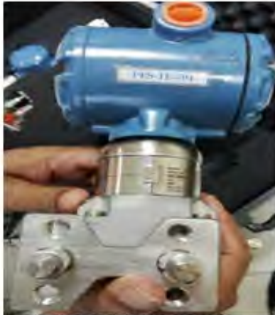
PRESSURE MEASUREMENT TRANSMITTER Maker: ROSEMOUNT Model: 305151CD12A12A12A1AQ4
