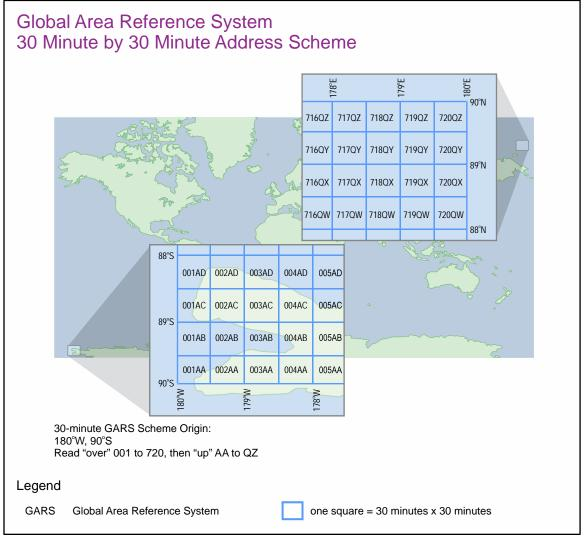
Figure D-1. Global Area Reference System 30 Minute by 30 Minute Address Scheme
