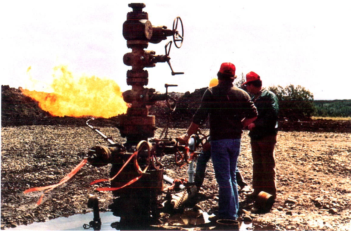
Canadian Hunter et al gas well flare in Elmworth Deep Basin, Alberta. This well location #10-27-70-11, W6M produces from the Falher zone, with a current capability of 12.5 million cubic feet per day.
