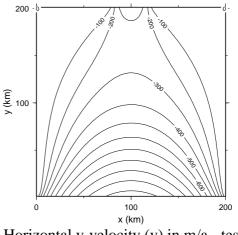
Horizontal y-velocity (v) in m/a - test 6
