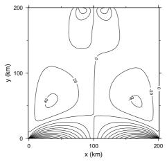
Horizontal x-velocity (u) in m/a - test 6
