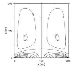
Horizontal x-velocity (u) in m/a - test 1
