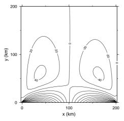
Horizontal x-velocity (u) in m/a - test 3
