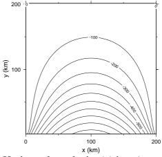
Horizontal y-velocity (v) in m/a - test 4
