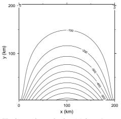
Horizontal y-velocity (v) in m/a - test 3
