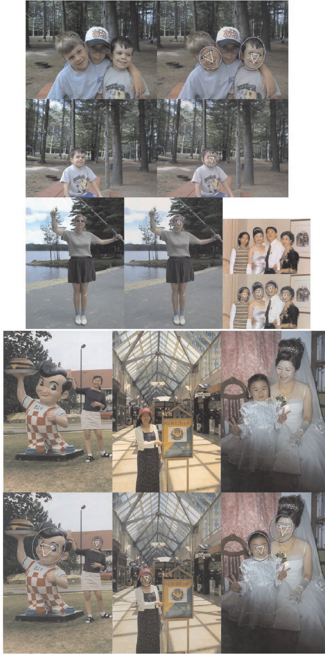
Fig. 15. Face detection results on a subset of seven family photos. Each image contains cluttered background. The detected faces are overlaid on the color-compensated images. False negatives are due to extreme lighting conditions and shadows. Note that the bias color in the original images has been compensated in the resultant images.
