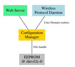
Figure 2: A simple architecture for enforcing per-UID access controls on data stored in an EEPROM
