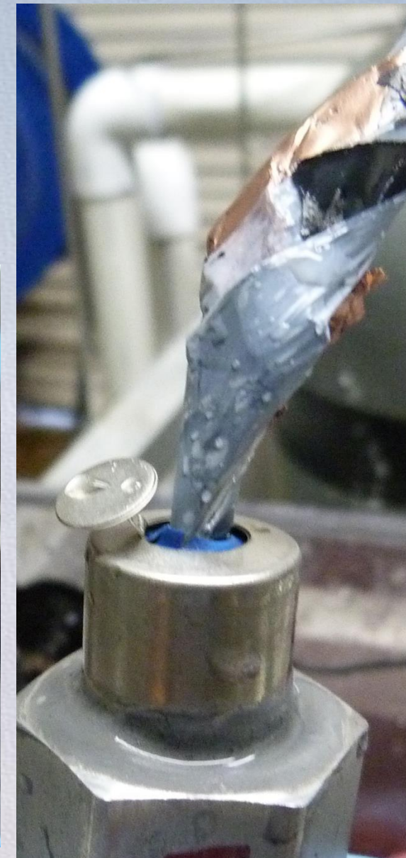
Bottom vent disk separates completely
