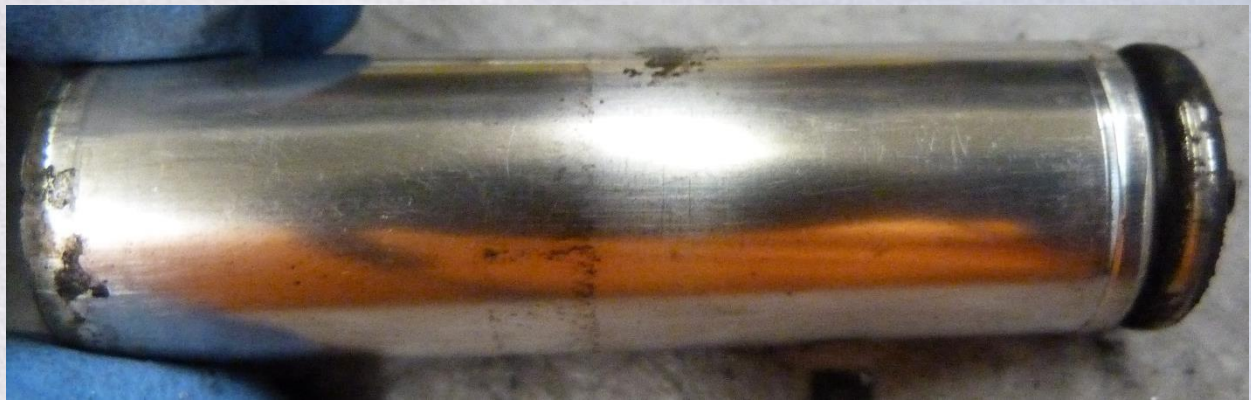
Spin groove is stretched
