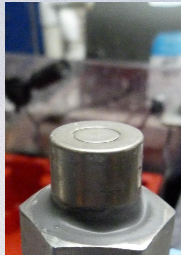
Bottom vent disk separates completely
