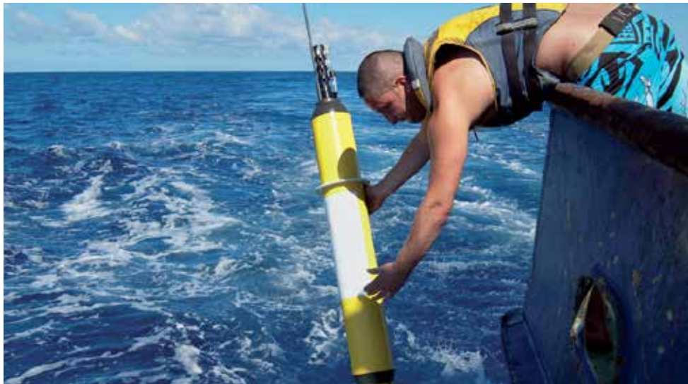
Figure 4.1 Since the early 2000s, thousands of robotic Argo floats have collected data enabling scientists to measure how the ocean has warmed and expanded.
