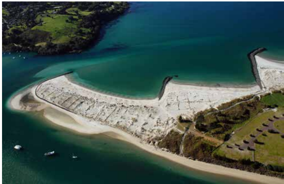
Figure 5.2 Omaha Beach north of Auckland is particularly prone to erosion. A severe storm hit in 1978, destroying the old sea wall. An Act of Parliament was passed for emergency remedial work including the construction of rock groynes and sand renourishment.
