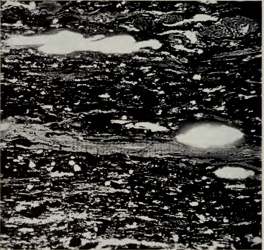
FIG. 11. A portion of a thin section of a block of Herrin (No. 6) coal in the mine of the Clarkson Coal and Mining Co., Nashville, Washington Co., Ill., illustrating the opacity of the groundmass of durain. The section is sufficiently translucent so that the coal represents semi-splint rather than true splint or durain.
