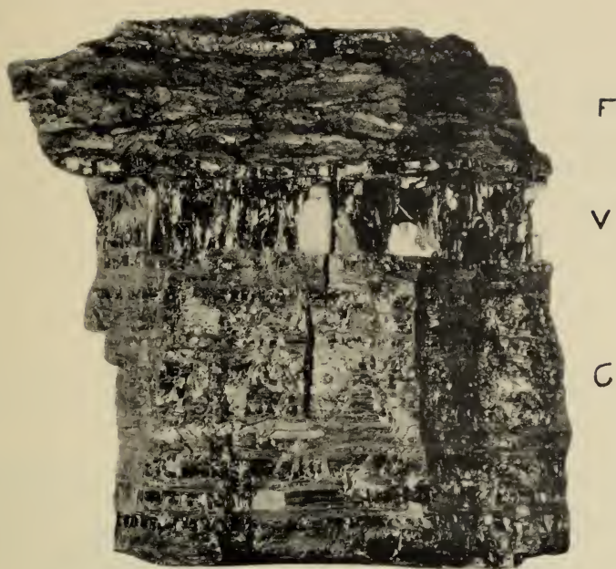
FIG. 1. Herrin (No. 6) coal, Orient No. 2 Mine, Chicago, Wilmington and Franklin Coal Co., W. Frankfort, Ill., showing Fusain (F), Vitrain (V), and Clarain (C) bands.
