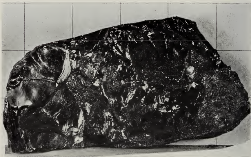
FIG. 6. Horizontal broken surface of a band of vitrain in coal from Herrin (No. 6) bed in the mine of the Midland Electric Coal Co., near Farmington, Fulton Co., Ill., illustrating the conchoidal fracture. (Net is 2 inches square.)
