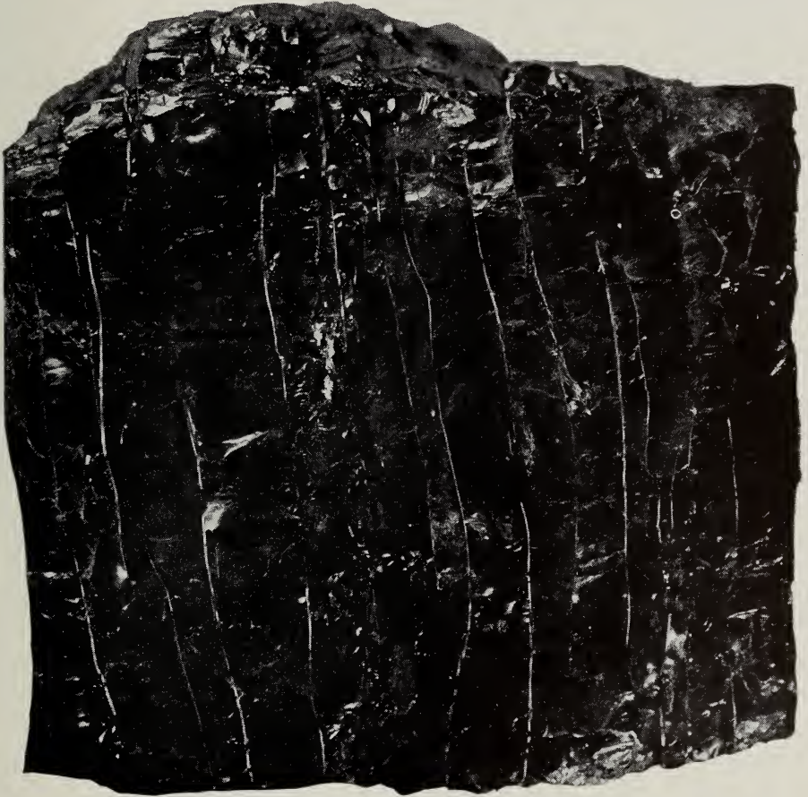
FIG. 7. Horizontal fracture surface of a band of vitrain in coal from one of the Brazil Block beds in Clay Co., Ind., illustrating the character of the fracture and the characteristic kaolinite-filled shrinkage cracks.
