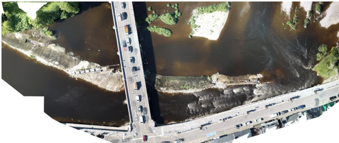
Figure 3.1.13 Fermoy weir a) 2016 (fully intact weir); b) 2018 (initial breaches on RHS) and; c) 2019 (full weir breach on RHS with mimicing of ‘rock ramp’ facilitating migratory fish passage).
