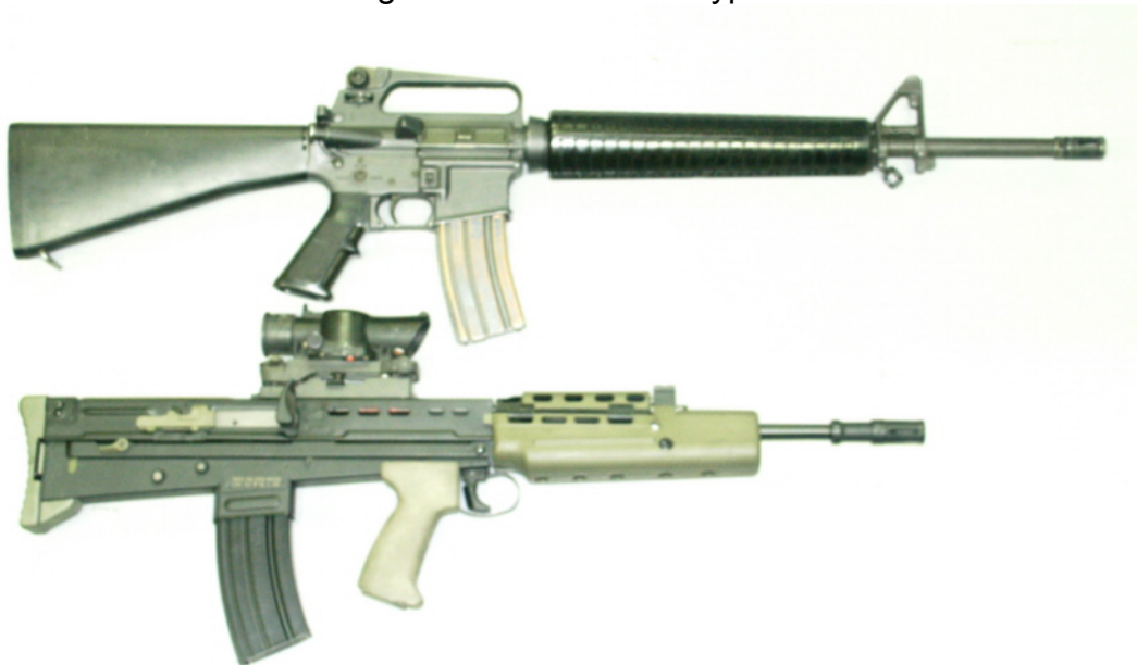
The photo above shows the M16 (top) and the L85: despite its shorter overall length, the L85 has a slightly longer barrel
