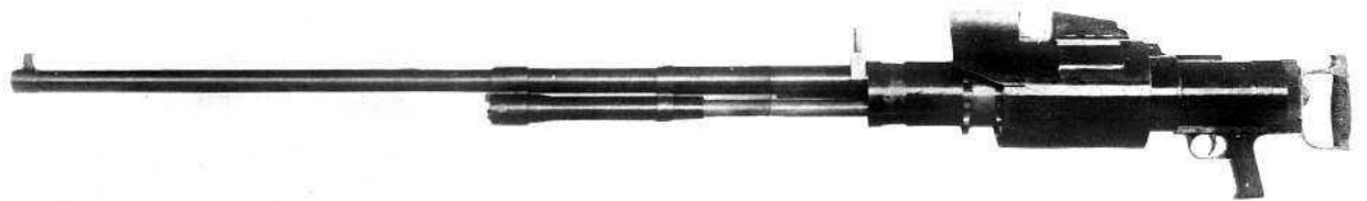
20 mm experimental ShVAK-type cannon TsKBSV-75
