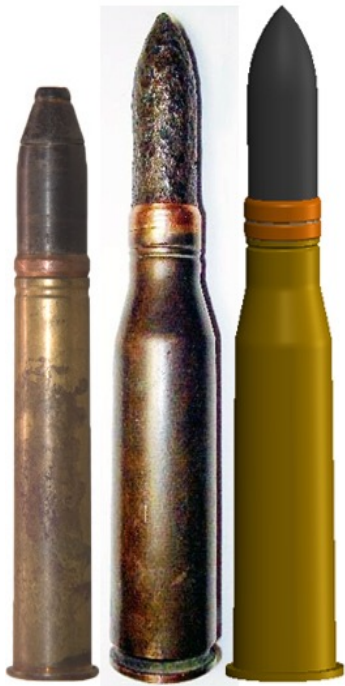
Russian cannon cartridges of the 30's - 20x99R ShVAK, 20x110, 20x110R (the 3d model)
