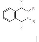
DiHepP consists of at least 80% of methylhexyl phthalate. Therefore the linear backbone is predominantly C6. The methyl group branching can be found on different C positions of the hexyl backbone chain.
