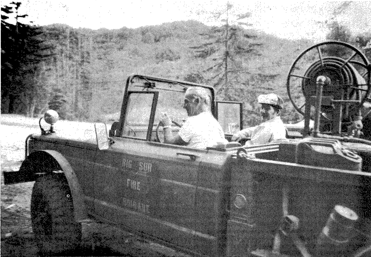
BIG SUR Brigade firemen Don Krausfeldt and Tom Sanders are shown in the Fire Brigade's new "first out" unit, a fast attack jeep with a 140-gallon slip-on pumper. Photo by Paula Walling.
