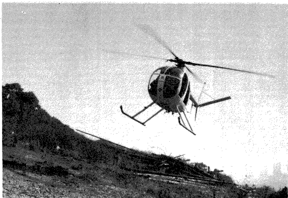
DROPPING REDWOOD POLES at the landing site, ARIS helicopter pilot Steve Sullivan swoops in and out of the canyon behind Willow Creek Basin in less than three minutes per load. The salvage timber was inaccessible by traditional logging methods and through the helicopter lift, fire hazard was reduced considerably. Photo by Kathryn Farmer.
