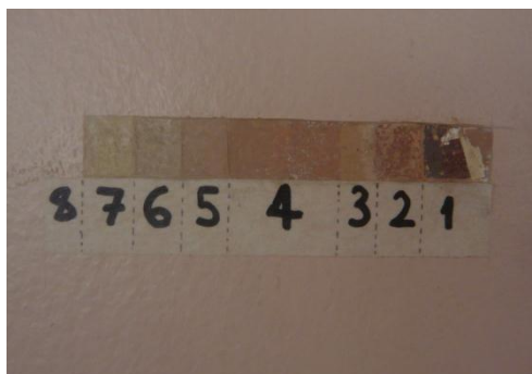
Color survey conducted during the 2009 interior restoration of the La Roche House – Dining room
