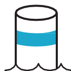
MOORING BUOY WHITE WITH BLUE BAND MAY SHOW WHITE REFLECTOR OR LIGHT
