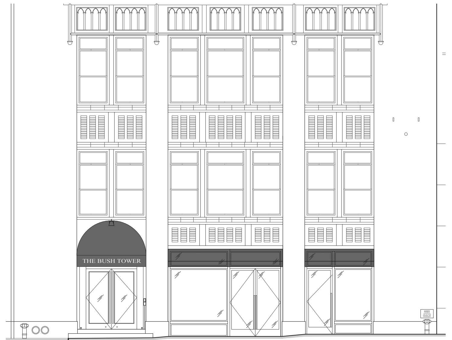
BUILDING ELEVATION OF PROPOSED STOREFRONT
