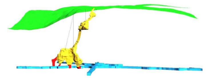
Figure 2: A stope section showing the areas in red and gold requiring backfill.
