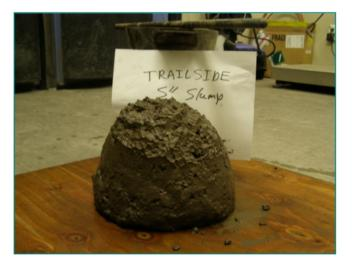
Trailside Sample Slump Test
