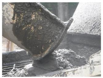
Figure 1: Paste backfill entering the pump hopper.
