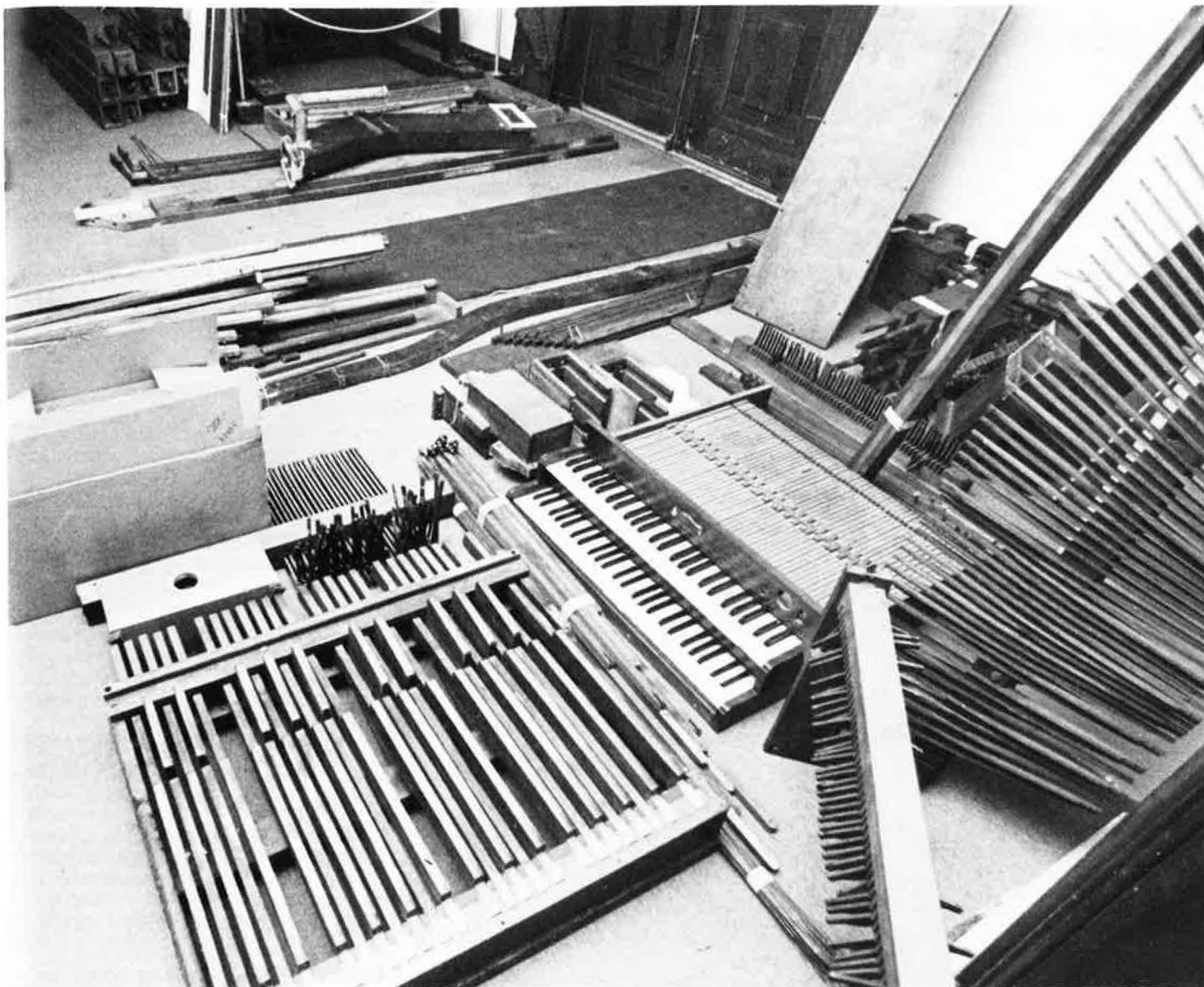
Photographed in Sag Harbor as it was disassembled, the mechanism of the 1845 Erben/1872 Earle & Bradley shows marked differences in construction techniques of the two builders when examples are closely examined in person. At the right, Erben's long backfall for the Great key action is a tour-de-force of superior craftsmanship, while Earle's competent square rail for the Swell key action appears in the right foreground; Earle's complex Swell action is seen in the pre-restoration photograph reproduced below.
