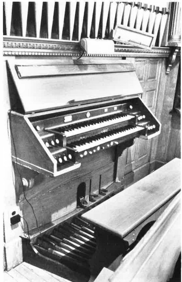
The keydesk of the Earle organ in Island Pond, Vermont, is original though the case is altered. Couplers are by pairs of off/on pistons located at the bass end of the Great keyslip.
